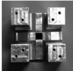
Figure 9: Top view of the concentrator receiver after lamination process.
