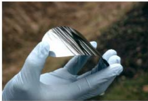
First attempts towards 30 – 50 \mu\text{m} thin and lightweight space solar cells on Ge are under development.
