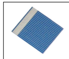
Figure 1. Small area cell cut from a 30X concentrator cell
