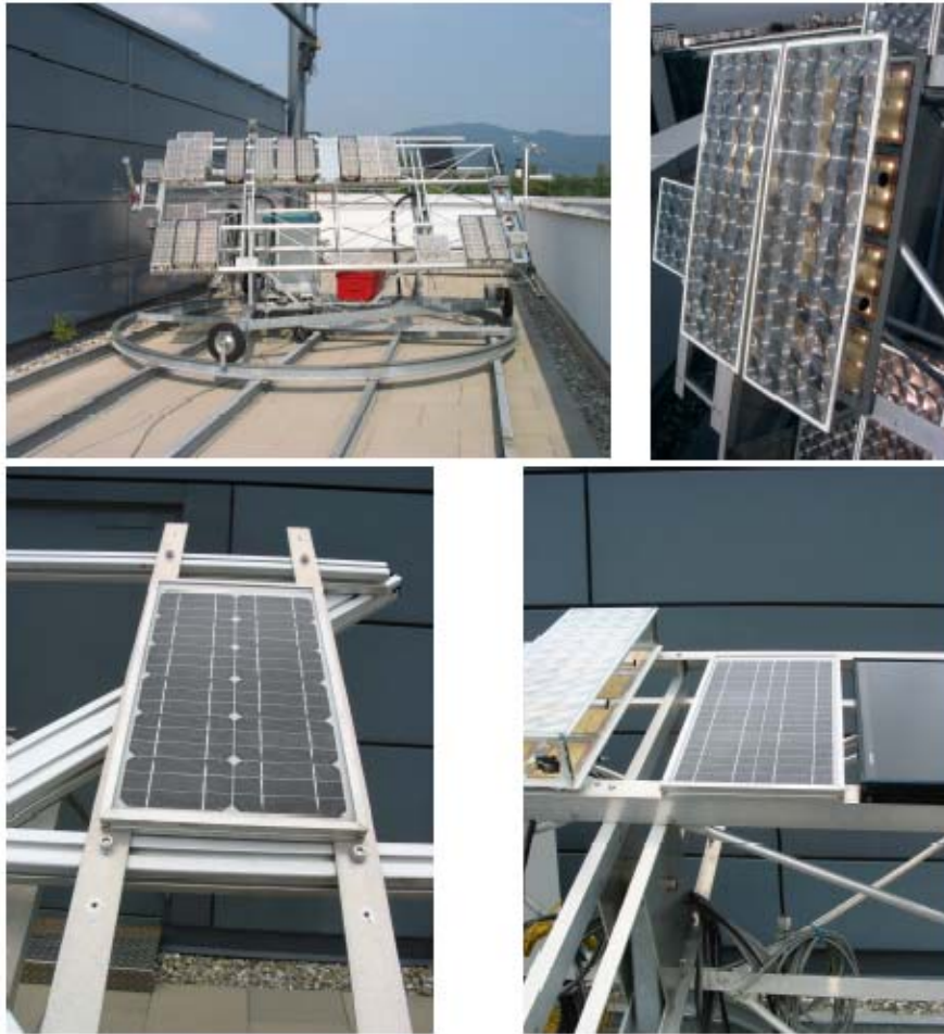
Figure 1: Photograph of the outdoor test set-up on the roof of Fraunhofer ISE in Freiburg. Top left: total view of the tracking unit with several FLATCON™ modules mounted on it. Top right: Detailed view of two FLATCON™ modules mounted on the tracker. Bottom left: fixed flat plate module. Bottom right: flat plate module mounted on the tracker.
